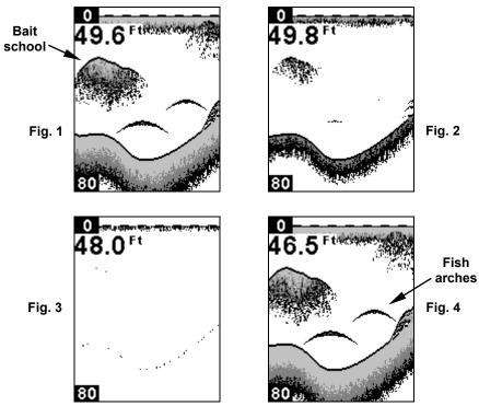
These figures show results of different sensitivity levels on the same location. Fig. 1: Sensitivity at 85 percent, determined by Auto Sensitivity. Typical of full auto mode. Fig. 2: Sensitivity set at 71 percent. Fig. 3: Sensitivity set at 47 percent. Fig. 4: Sensitivity set at 90 percent.
